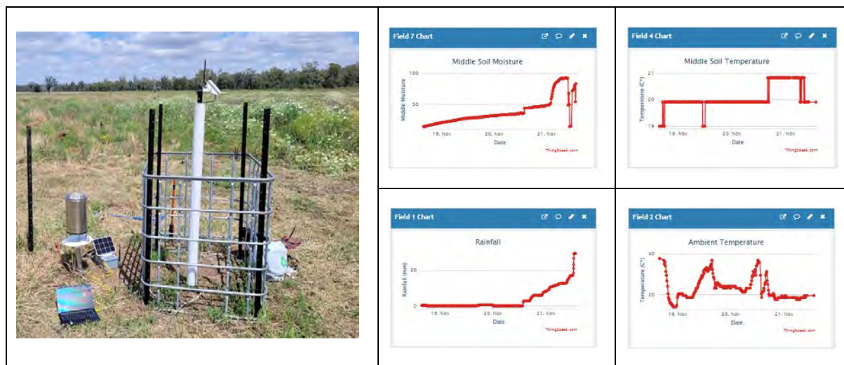
Figure 1.2: Left: a sensor node installed in Narrabri. Right: data generated for soil moisture, rainfall, soil temperature and ambient temperature.
